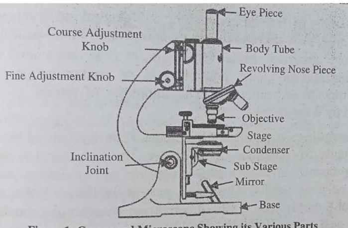
Figure 1: Compound Microscope Showing its Various Parts
